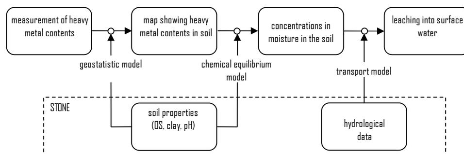
Figure 1. Schematic representation of the heavy metal leaching model
